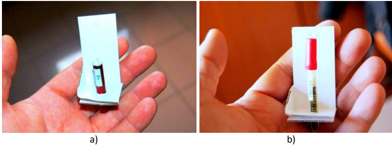
Figure 1. Example of the tracer gas sources a) and samplers b)
