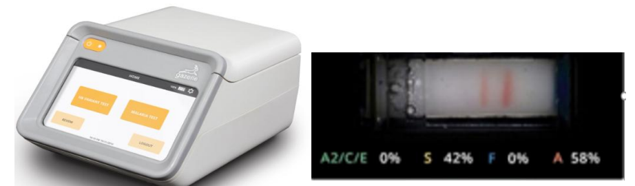
Figure 2- Gazelle equipment and display showing the HbS quantification (HbS=42%).
