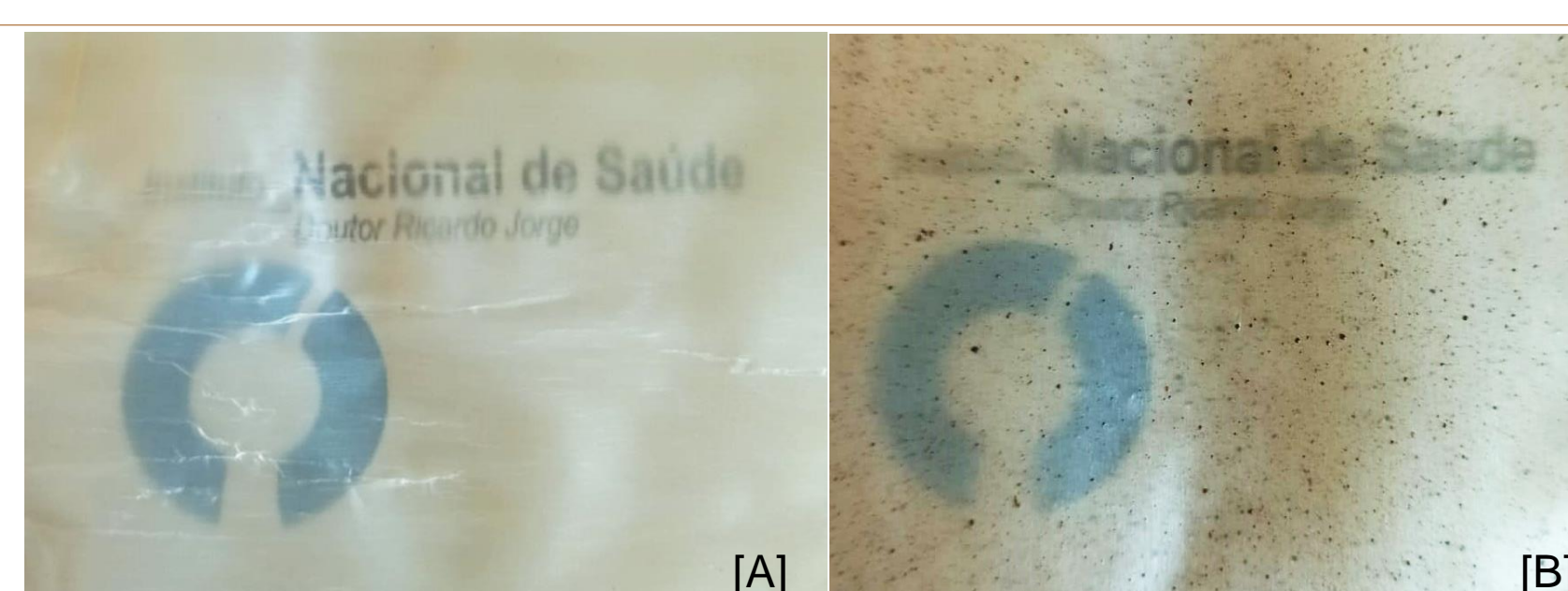
Figure 2. PLA-based active packaging with 3% of pomegranate peels extract (PLA/3PPE) [A] and with 3% of pomegranate peels (PLA/3PP) [B].
