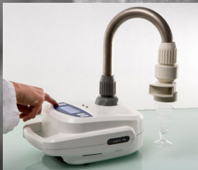
Fig. 2 - Equipment used for air samples collection to apply molecular identification
