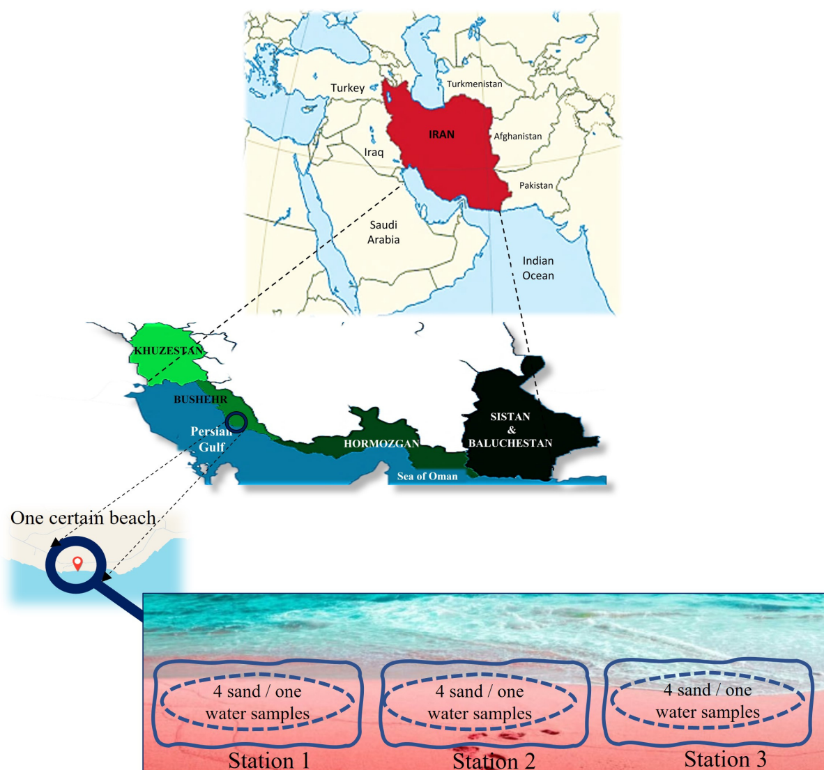
Figure 1. The provinces selected for sampling are located along the coastlines of the Persian Gulf and the Sea of Oman. Each beach was divided into three stations, and from each station, four sand samples were pooled into a single sample, resulting in one sand and one water sample. Finally, 39 sand and 39 water samples were taken from 39 stations. Sampling was performed from sand and water from May to July 2023.
